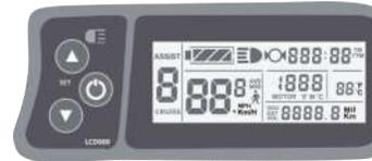
The metric units will be set after finishing setting wheel diameter, KM/H and Km flash. Hold or button shortly and select the three metric units of speed, mileage, and ambient temperature in synchronization.
