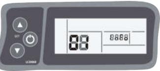
Electronic control system failure will display (flashing) fault code. Once the fault was removed, it automatically exits from the fault code display interface.
