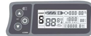
Hold or button shortly to switch 1-5 file gear. Gear 1 is for the minimum power, gear 5 is for the highest power. Each startup will automatically restore the gear shutdown last time (the user can set randomly). Gear 0 is without booster function.
