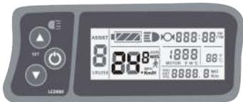
After power on for 5 seconds, hold and button at the same time, maximum riding speed KM/H and MXS flash, hold or button shortly to set the maximum riding speed (default
