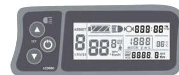
After power on for 5 seconds, hold and button at the same time, single trip riding time (TM) and single trip distance (DST) flash, hold button shortly, the content of both is cleared. If failed holding the button within 5 seconds, it will automatically return the display interface after 5 seconds, original content is preserved.
