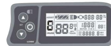
After the cruise function is turned on, the trip riding speed is greater than 7 km/h, hold button long and enter cruise, the CRUISE lit. Brake or hold any button to cancel.
