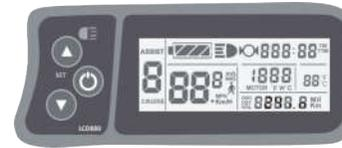
The wheel diameter will be set after finishing setting the maximum riding speed, wheel diameter specifications flashes. Hold or button shortly to set the specifications of wheel diameter. Select the range 6,8,10,12,14,16,18,20,22,24,26,700c and 28
