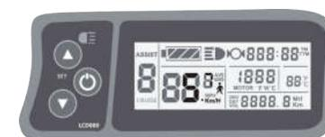
Hold button and flashes, the vehicle drives at the speed not more than 6Km/h. Release button, the function is invalid.
