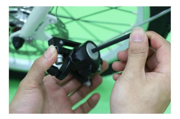
3. Fasten the brake device by the screw first. Then adjust the spacing between the brake device and disc brake by the hexagon socket. Ensure that there is no friction between the disc brake and brake device. The smaller spacing of both sides, the better the brake works.
