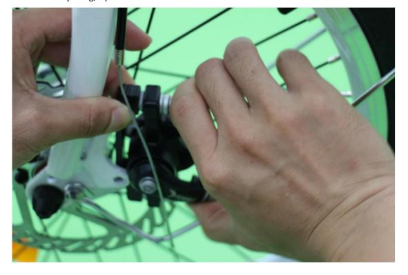
2. Adjust the firmness of the brake device by hexagon socket. Adjusting the firmness is to adjust the gap between the brake pads, getting them as close to the disc as you can without rubbing.
