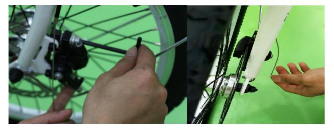
4. After adjustment, insert the brake cable to fix the screw.
