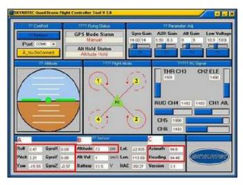
value you should set for 3 cell (11.1v) lipo is 10.9 if you want to completely drain your battery during flight. We highly recommended to keep the value to 11.1v in order to make sure your quadcopter will not crash once the low voltage warning kicks in and also your battery will have a better life cycle.
